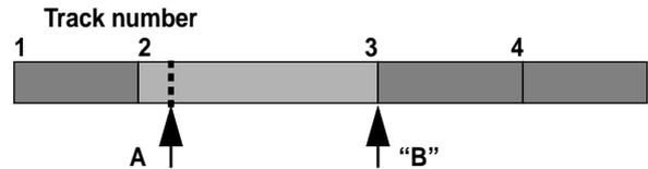
This provides a convenient way to delete from a marked point to the end of the track.
